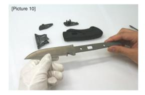
7 To assemble, carry out steps ① to ⑥ in the reverse order. When inserting the knock pins, be sure to insert knock pin A first and then insert knock pin B. To avoid accidental disassembly, make sure that each part clicks securely into place and are attached in the correct locations.
