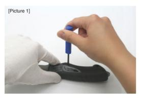
2 Next use the screwdriver to gently lift up and remove knock pin B. [Picture 2], [Picture 3].
