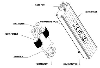
Connection of the battery tank FX1206 / FX1209 onto the cilinder Slide the bracket of the battery tank over the belt of the stabilizing jacket. Close the belt securely.
